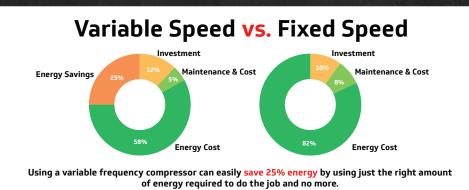
Sullivan-Palatek compressors with **Variable Frequency Drive (VFD)** dynamically adjust motor speed to match air demand, cutting power consumption. Key benefits include:
