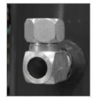
Lube Fill & Level Elbow
