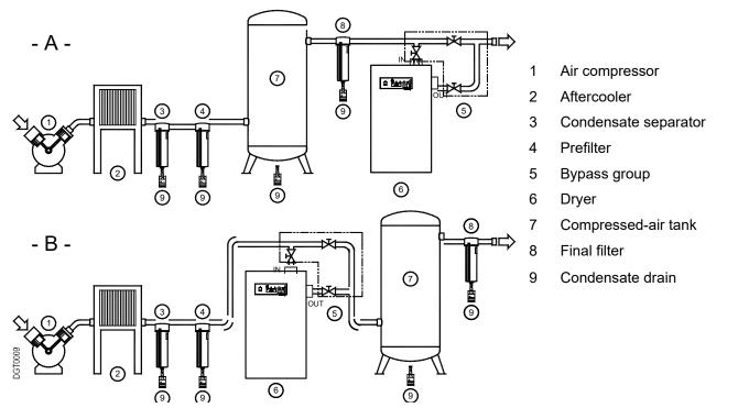
Installation **type A** is recommended when the total consumption corresponds to the throughput rate of the compressor. Installation **type B** is recommended when the air consumption constantly varies, with peak values which considerably exceed the throughput rate of the compressor. The storage capacity of the tank must be dimensioned in such a way that a possible short-term high air demand (peak air consumption) can be compensated.
