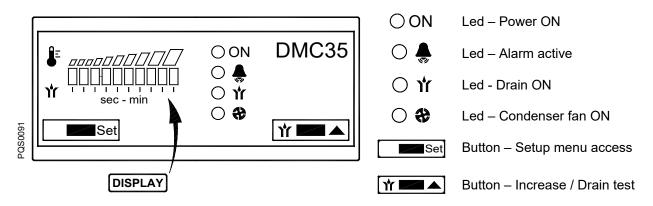
The DMC35 displays DewPoint temperature, controls the condenser fan activation, controls the timed drainer and keep record of the total hours of operation of the dryer.
