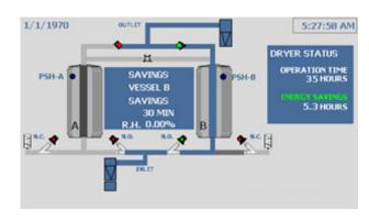
After this second Savings step, the controller will continue back to Step 1. Note that the Savings step function is only applicable if it has been enabled in **SETTINGS** (under the Energy Management option). To enable this, refer to the **SETTINGS** section of the manual.
