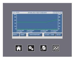
Pressing **HISTOGRAM** allow a real time trend line of the relative humidity of the dryer. At full a total of 80 minutes can be displayed.
