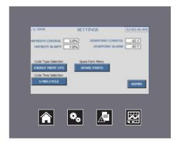
Within the **SETTINGS** function of the controller, the system can be configured based on several characteristics that will affect the operation of dryer:
