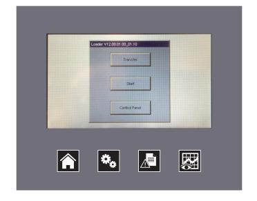
The **START** screen is only displayed for 3 seconds, after which, the **HOME** screen will be displayed and the controller will automatically begin its drying sequence.
