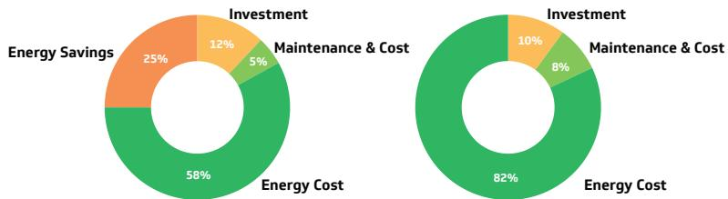
Using a variable frequency compressor can easily **save 25% energy** by using just the right amount of energy required to do the job and no more.
